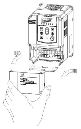
Removing the cover and the blocking board
