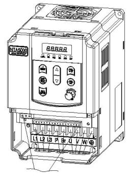
Wiring and divided by blocking board (Power wiring is under the control wiring)
