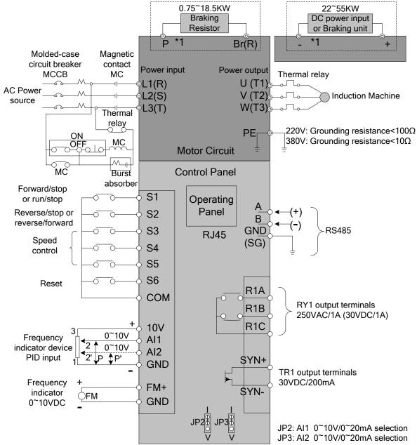
Note  $^*1$  Please refer to description of main circuit terminals (P, Br(R)) and specification of braking resistor for value selection.
