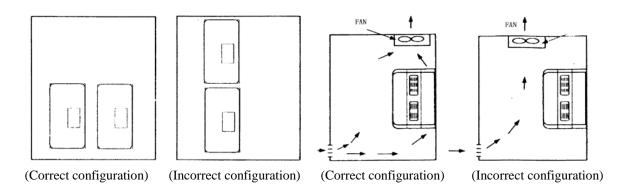
Place the inverter facing forward and its top facing upward to assist with cooling.
