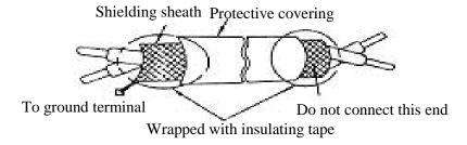
(C) Inverter Ground terminal must be connected to installation ground correctly and according to the required local wiring regulations.
