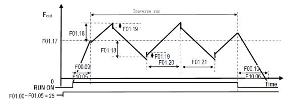
2. When traverse running, only the multi-function terminals can change upper deviation of the center frequency (F01.05=26 and breakover) or lower deviation of the center frequency (F01.00~F01.05=27 and breakover). But the commands of upper and lower deviation of the center frequency can't be used at the same time, and if they were used in the meantime, the frequency will maintain the original center frequency, please see the diagram as below:
