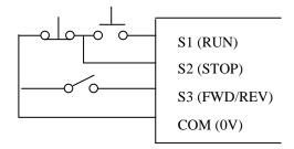
Wiring control sequence is as below:
