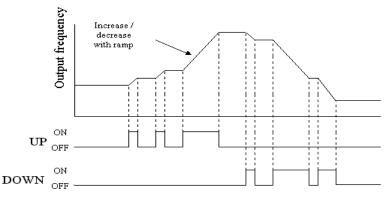
2. F01.07=0.01~5.00, and UP/ DOWN terminal ON, is equivalent to a step increase/ decrease at the increment frequency in F01.07. If UP/DOWN is pressed over 2 seconds, the original UP/DOWN mode is restored (Please refer to the following diagram)
