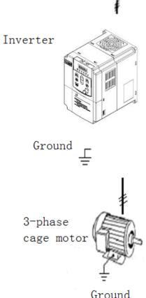
Making external connections should according to the following instructions. Check connections after wiring to make sure all connections are correct. (Do not use the control circuit buzzer to check connections)
