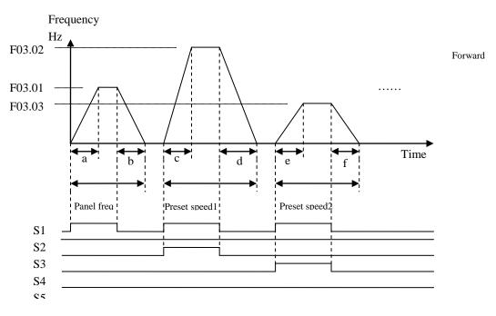
Mode 2: When the run command is continuous, calculate acceleration and deceleration time of each segment like this
