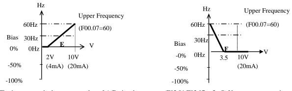
The inverter reads the average value of A/D signals once per (F02.01/F02.07 x 2mS). Users can set scan intervals according to possible noise interference in the environment. When the noise is serious, increasing the F02.01/F02.07, but the response time will increase accordingly.
