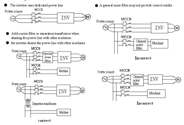
A noise filter in the output of the main circuit can suppress conducted noise. To prevent radiated noise, the wires should be put in a metal pipe and distance from signal lines of other control equipment should be more than 30 cm.
